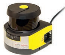
Safety scanner RSL420-S/CU416-5 with 10 individual switch- able field pairs. Maximal range 3m at 220° Item number M4061
